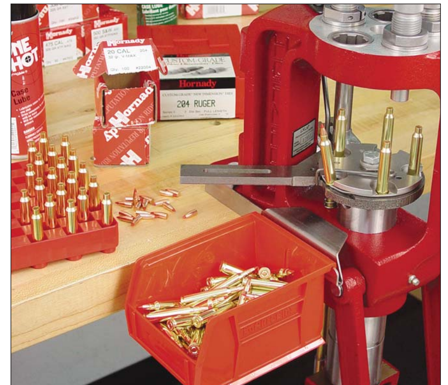
Here's the payoff to the 'pleasures of a progressive press'; a completed round on its way to the “collection basket” with each pull of the handle!
